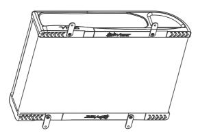
Step 2: Secure the enclosure with four screws.
